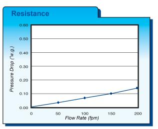
\*20" X 20" filter tested per ASHRAE 52.2, Test Aerosol KCl, Neutralized. This test data is based upon clean filter performance. All filters increase in efficiency with dust loading.
